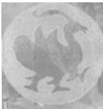
Fig. 5. An example of image recording. The color red was developed in the irradiated parts after diazotization followed by treatment with naphthol AS on the polymer surface.
